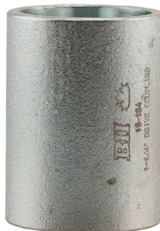
Available in steel and stainless steel and are used during well point installations. They are designed to withstand the impact force required to drive a well point into the ground. They have a specific design to ensure that the weight is not carried by the threads.
