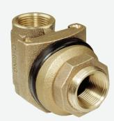
A Pitless Adapter sits inside your water well below the frost line. It takes the water from your well, turns it 90 degrees, and sends it out the side of the casing into the service line, and into your house. They also create a watertight seal.
